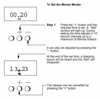
NOTE: If necessary the minute minder can be cancelled before the bleeper sounds by pressing the "+" and "-" buttons together until 0.00 appears in the display window.
