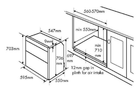
1. When installed in a typical 600mm deep built in housing unit, the false back should be removed from the housing unit to provide the necessary depth for
