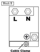
If your appliance is fitted with the terminal block below, for multiphase appliances please remove the links from terminals L1, L2 and L3 only. Leave neutral links fitted to terminals N4 and N5.
