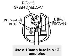
As the colours of the wires in the mains lead for the appliance may not correspond with the coloured markings identifying the terminals in your plug, proceed as follows:
