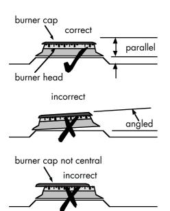
Burner caps and heads must be repositioned correctly so that they sit squarely on to the hob as shown on the the left.
