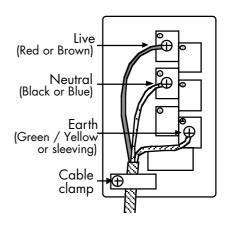
Sufficient cable should be used to allow the cooker to be pulled out, but must hang clear of the floor so it does not become twisted or trapped when the cooker is pushed back.
