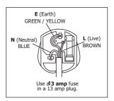
The wires in the mains lead are coloured in accordance with the following code:
