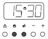
To set the programmer to manual operation at any time (cancelling any automatic setting), press the *cook time* and *ready time* buttons simultaneously. The programmer must be set to manual before the appliance can be used manually.
