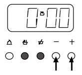
Press the *cook time* and *ready time* buttons <u>simultaneously</u>, and keep the buttons depressed. Use the *plus* and *minus* buttons to set the time of day, eg; 12.00.
