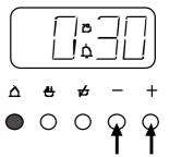
Press the *minute minder* button, then use the *plus* and *minus* buttons to set the required time.
