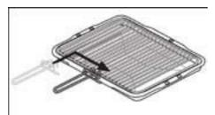
The handle is designed for removing / inserting the grill pan under the grill when grilling.
