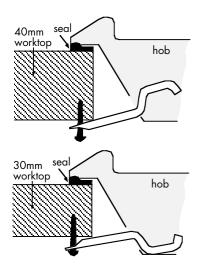
The screws should be tightened just sufficiently to secure the hob and pull the top pressing flush with the worktop.
