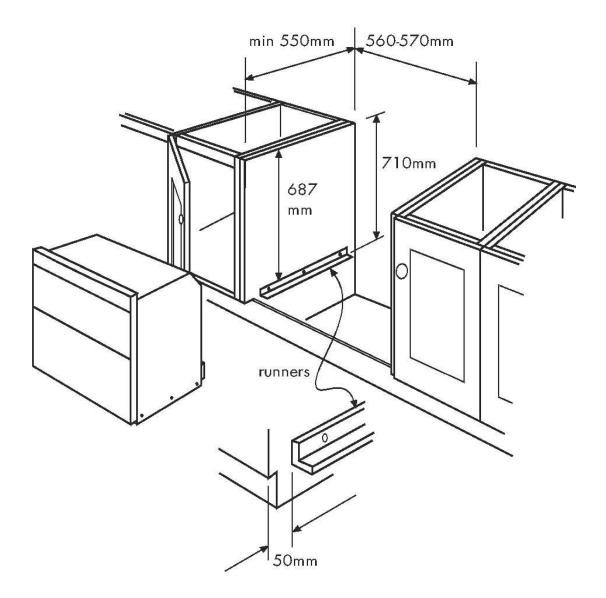
*Method 2:* Housing unit with internal height less than 710mm Shown without fixing kit
