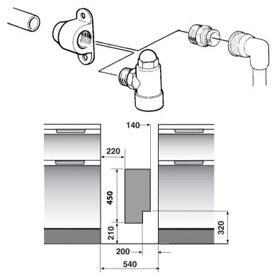
Connection to the cooker should be made with an approved appliance flexible connection to BS 669. A length of 0.9 to 1.25m is recommended. The length of hose chosen should be such that when the cooker is in situ, the hose does not touch the floor.
